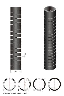
HDPE slotted and normal pipes designed to collect the leachate and the biogas from landfills as well as draining in constructions works.
