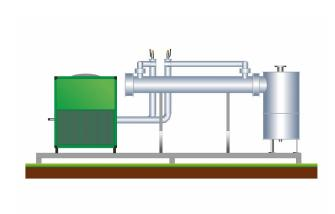
The system includes the equipment and instruments needed for initial treatment of biogas entering the motors to eliminate moisture content and, at the same time, reduce hydrogen sulphide content. It can be installed as standard equipment of the inlet system or assembled separately on a specifically designed chassis. The main components of the system are the biogaswater heat exchanger, the chiller and the condensate collection and discharge equipment.
