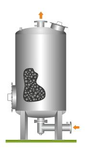
Activated carbon filters are installed for contaminants removal from biogas/air and odour control. Selection of the most suitable activated carbon is based upon the application and the contaminant to be removed (typically, hydrogen sulphide H2S, or siloxanes).
